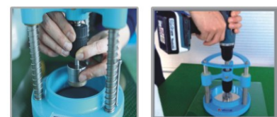
How to mount a drill bit
