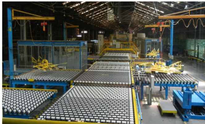
Jib crane with Horizontal vacuum lifter
